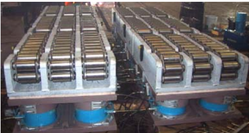
Six, 1,250 Ton load capacity Rollers with Rams in pre installation tests.
